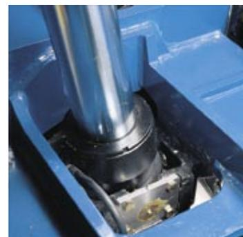
**Strong oscillating mounting design lets the lifting cylinders move freely, with no twisting forces on cylinder rods.**
