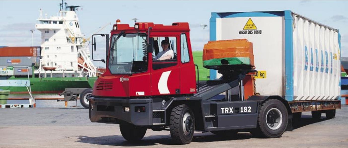
Ease of maintenance; well protected side compartments with big and easy opening covers for pneumatics and hydraulics.
