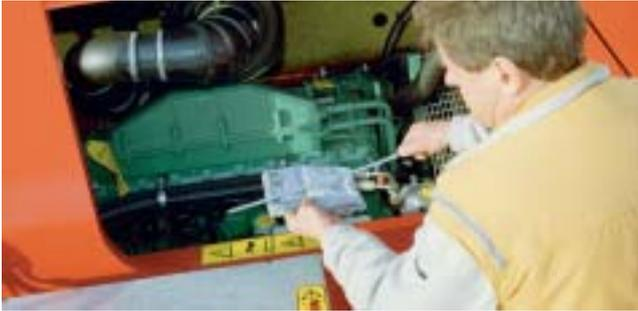
points and inspection covers for easy access are a good start. For major overhauls the driveline is easily accessible thanks to the tilting cab.
