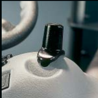
Joystick control or a mini steering wheel in the arm rest mean great ergonomics for the driver.
