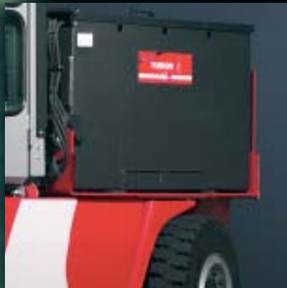
Battery replacement system where the battery either slides out along tracks, or has slots for forklift, increases the truck's operational availability.
