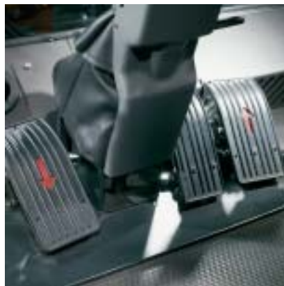
Dual pedals for forwards and backwards let the driver manoeuvre the truck quickly and safely, and ergonomically.
