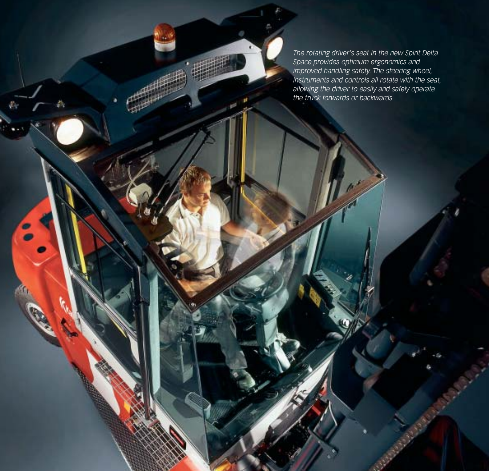
Spirit Delta has undergone further development to provide extra width for more space for installing additional equipment.
