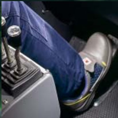
Hydraulic inching is available as an option, controlled by the KCS. Inching allows precision operation even while maintaining high engine speeds for efficient lifting.
