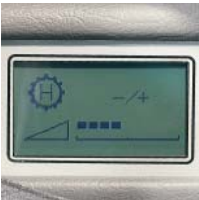
The engine brake can be adjusted to one of nine settings, from insignificant to full force.
