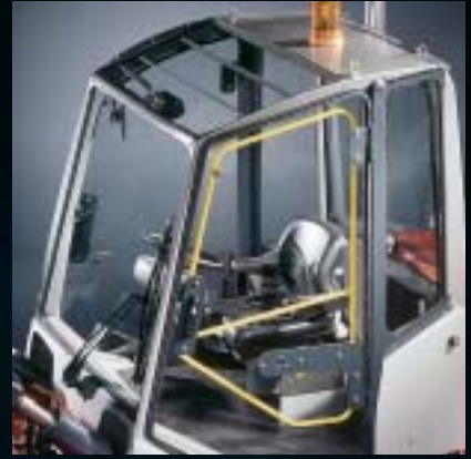
FlexCab is a robust and efficient driver environment that can easily be adapted to a FlexGuard safety cage.
